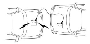
3. Remove the jumper cable from the positive (+) terminal of the booster vehicle's battery.
